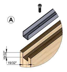
Groove bottom of door to suit 42-1 channel size19/32 " x 19/32") cut channel to suit door. Fix with No. 6 x 3/4" countersunk woodscrews- fig. A.
